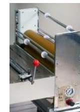
Air pressure nip rollers
