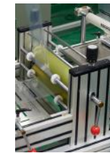
Spring-coil pressure nip rollers
