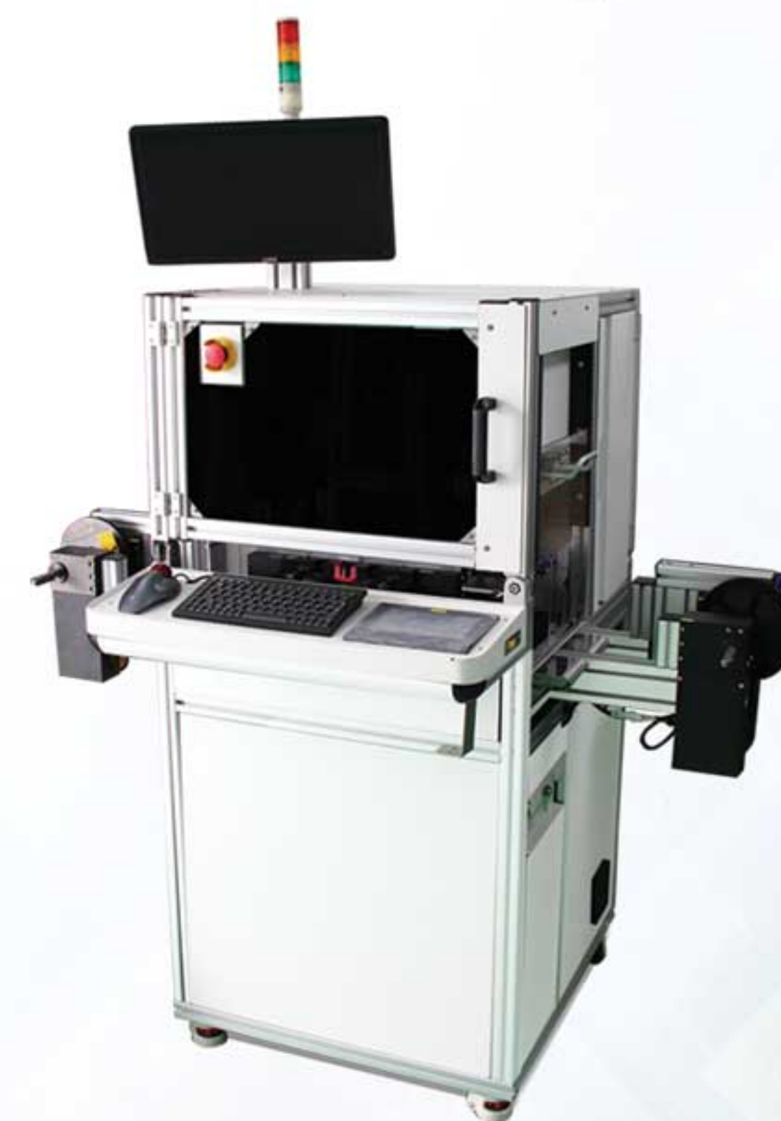
AutoVIT Reel to Reel Vision Inspection
